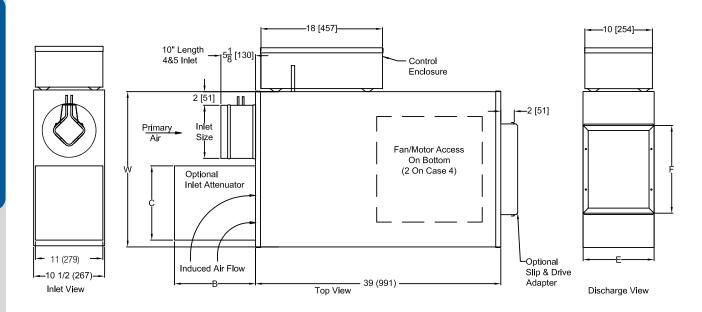
The standard location for control enclosure is Left Hand on model XG-FCL. Looking in the direction of airflow, the control enclosure is on the left.
