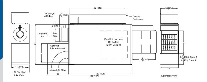
The standard location for control enclosure is Left Hand on model XG-FCL. Looking in the direction of airflow, the control enclosure is on the left.
